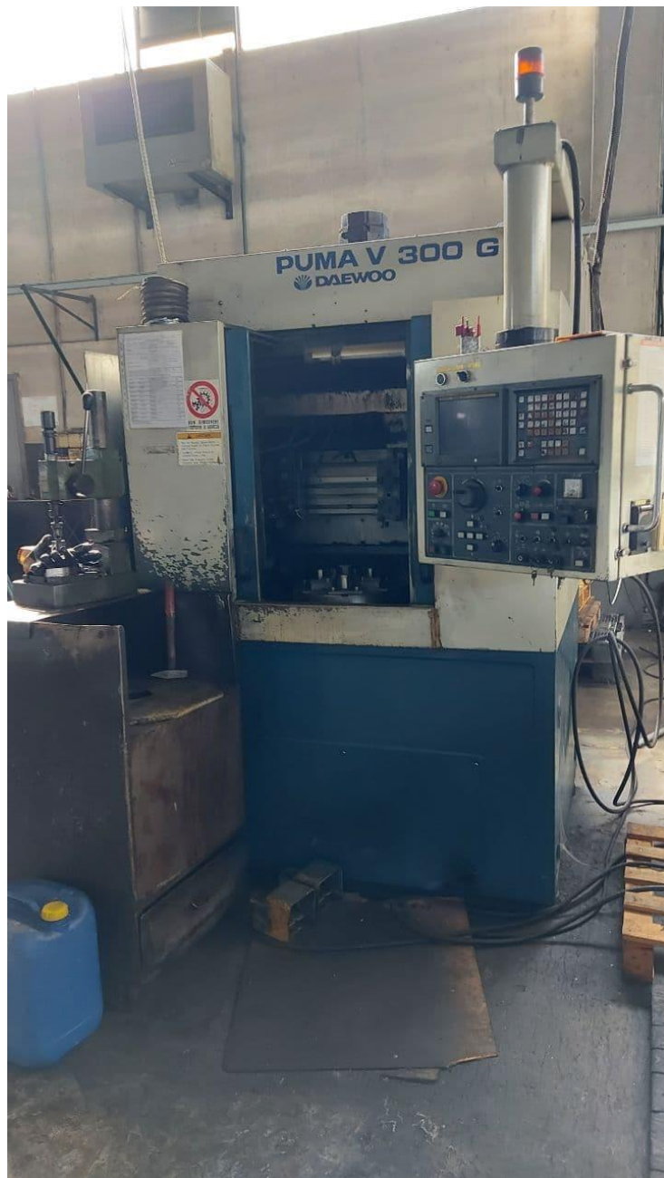
Puma V300G machining centre with double carriage
